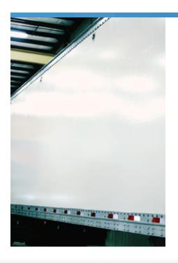
STRICK'S FRC PANELS are hydrophobic and will never "wick" water, preventing weight increases and de-lamination. Carriers can now enjoy the advantages of snag-free interiors, ultimate durability, the repairability of fiberglass, and lower tare weights. These characteristics, combined with many other high-end Strick van design specifications, are assembled in our ultra-modern facility in Monroe, Indiana.
