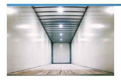
**FAMILIAR MATERIALS** come together in a new revolutionary process to make up the Strick FRC van. The FRC features side-walls that are pultruded with a moisture-resistant foam core that is 100% recyclable. No other trailer on the market today delivers this unique and compelling combination!
